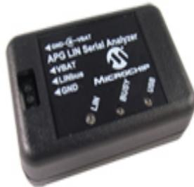
The LIN Serial Analyzer development system enables a Personal Computer (PC) to communicate with a LIN (Local Interface Network) bus as a network debug and analysis tool. The LINSAs can reside on the bus as a master, slave, or non-intrusive snoopers. The included PC program uses a graphical user interface to enter and display message frames occurring on the target bus.
