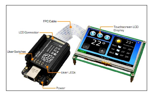
Figure 8: Connecting the BB-View, BeagleBone Black and the LCD Module
