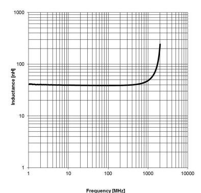
DESCRIPTION Projection **WE-CAIR Air coil** Würth Elektronik eiSos GmbH & Co. KG EMC & Inductive Solutions Max-Eyth-Str. 1 Order.- No. 74638 Waldenburg COMPLIANT SIZE Germany Tel. +49 (0) 79 42 945 - 0 744912139 www.we-online.com A4 2014-03-24 SSt 1.0 HBH eiSos@we-online.com REV Size: 4248 DATE CHECKED
