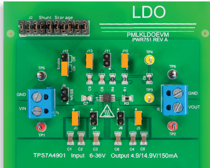
Figure 6. TPS7A4901 LDO board: jumpers set-up for Test#1
