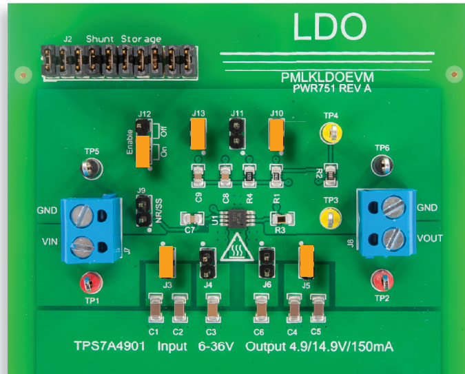
Figure 6. TPS7A4901 LDO board: jumpers set-up for Test#1
