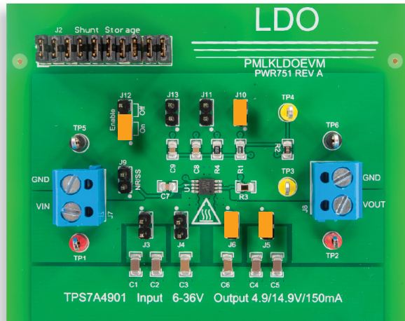
(a) TPS7A4901 LDO regulator under test
