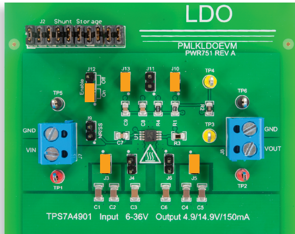
(a) TPS7A4901 LDO regulator under test
