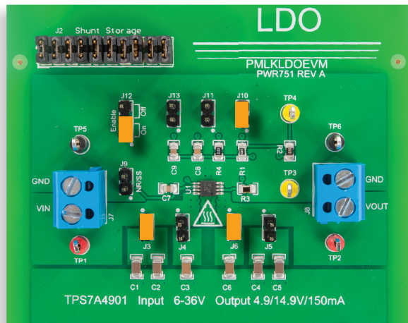
(b) TPS7A4901 LDO regulator operating as line injector
