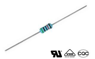
A metal glazed film is deposited on a high grade ceramic body. After a helical groove has been cut in the resistive layer, tinned electrolytic copper wires are welded to the end-caps. The resistors are coated with a light blue lacquer which provides electrical, mechanical, and climatic protection.
