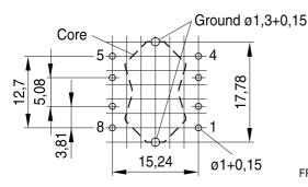
Hole arrangement View in mounting direction
