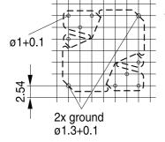
Hole arrangement View in mounting direction
