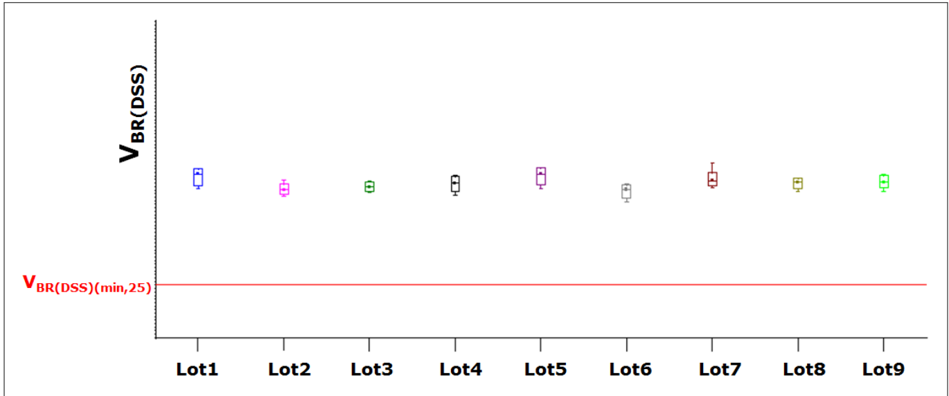
Figure 8 Example of production distribution for V_{BR(DSS)}
