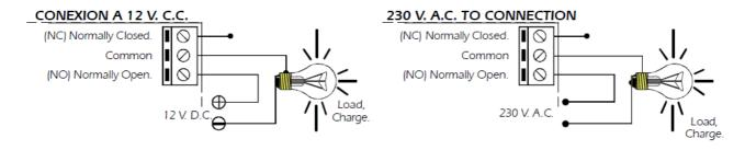
During the operating, and according to its load, it is possible that a fluctuation appear and/or an incorrect output operating. If it is the case, you have to install a circuit against sparks (resistor or capacitor) between both relay contacts used for the connection. (see the drawing)
