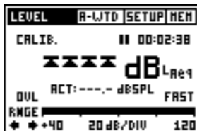
Fig 3.4 SPL Panel with Overload
