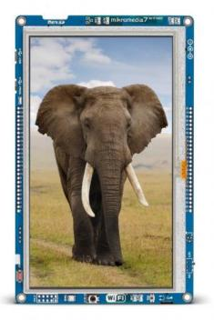
Vivid 7" 800x480px touch screen and over 30 on-board modules, including Ethernet, WiFi and ICDI debugger all packed onto a single board. Everything is orchestrated by the mighty <u>STM32F746ZG</u> ARM Cortex-M7 microcontroller family.
