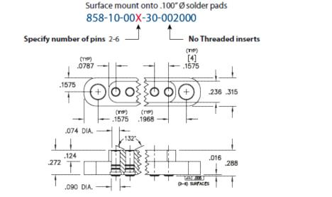
Spring-Loaded Header Vertical Mount SMT Target with Concave Face Single Row Surface Mount Plating Code: 10 Shell Plating: 10 µ" Gold over 100 µ" Nickel Packaging: Packaged in Tubes
