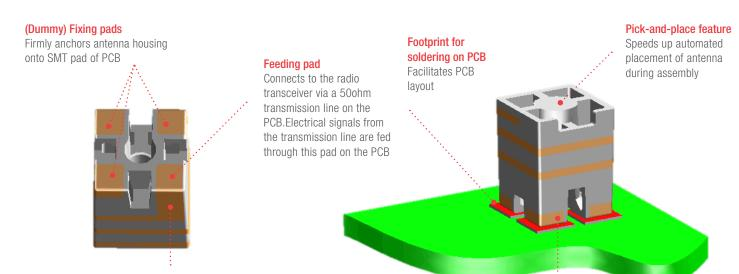
**Gold (Au) over Nickel (Ni) radiator traces** Act as transducers that convert unguided electromagnetic waves to guided electromagnetic waves and vice versa
