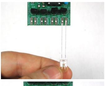
Next is the IR LEDs. Start with **LED1**, a clear IR led. Like the small indicator LED, it has polarity. Make sure the longer, positive lead is on the right, as shown.
