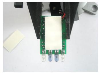
Place the doublesided foam sticky on the circuit board. Remove the other side and press the battery holder on.
