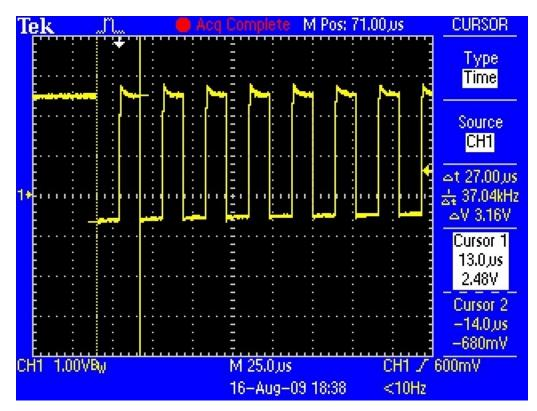
You can measure the frequency of the IR pulses. As you can tell by the cursors and the measurements on the side, the frequency is about 37.04KHz
