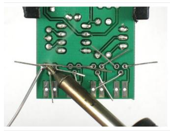
Turn the PCB over and solder in all the transistors. Then clip the wires.
