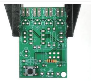
Next is the 1.0 kilo ohm resistor **R5**. This is the brownblack-red striped part. This resistor sets the brightness of the little indicator LED. Resistors are symmetric, so it can go in either way.
