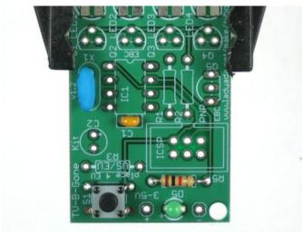
Next, place 2 components. The ceramic oscillator and the 8-pin socket. The oscillator has 3 pins and is symmeteric. The oscillator is the timeclock for the microcontroller, making sure that it is performing its functions at the correct speed.
