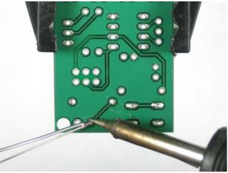
Turn the PCB over and solder both leads of the LED.
