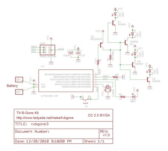
Now we use one pin, PB0 to drive Q5 the PNP which connects the bases of the driver NPNs with a path to VCC.
