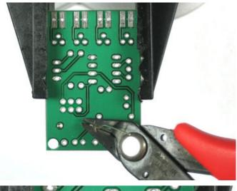
Use the diagonal cutters to clip off the resistor legs so that only the solder points remain.
