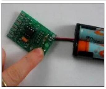
Test the kit now by putting two good AA batteries into the holder. The green indicator light should blink to show that the microcontroller is functioning properly. If you don't get a blinking light check the batteries, make sure the indicator LED is in correctly, and that the chip is in the right way.
