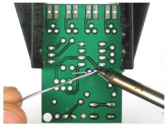
Solder and clip the ceramic capacitor part.
