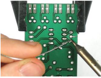
Solder the rest of the points then clip short the legs of the oscillator.
