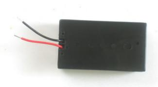
Use your soldering iron to 'tin' the wire, melting solder into it to keep the wire from fraying.
