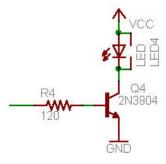
The IR LEDs have more than 100mA going through them. This is way more than a microcontroller pin can supply (usually 20 to 40 mA max!) so we use a 'driving' transistor. These NPN transistors amplify the power of a microcontroller pin and are designed to turn off currents of over 100mA. When the base pin is pulled high (though the base resistor) the transistor turns on and the LED turns on too. When the base pin is pulled to ground, the transistor turns off and no current passes through the LED.
