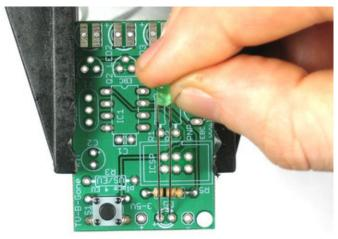
Now it's time to place the small indicator LED **LED5**. LED's are not symmetric and must be placed correctly in order to work. You'll notice one leg of the LED is longer than the other. This is the *positive* leg. The positive leg goes into the hole with a + next to it. In the picture shown, its the left hole.
