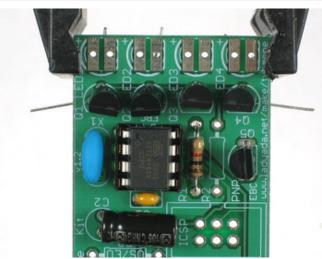
Next are the four NPN (2N2222) transistors **Q1 Q2 Q3** and **Q4**. These are the devices that turn on and off the high power IR LEDs. The microcontroller doesn't have the capability to provide a lot of power directly to the LEDs so these transistors assist it.
