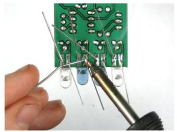
Flip over the PCB and solder it to the bottom.
