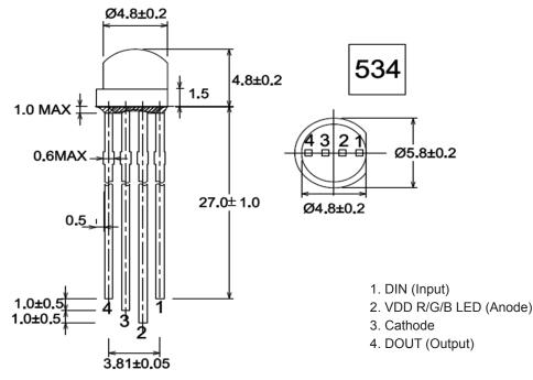
Dimensions : Millimetres Tolerance is ±0.1mm
