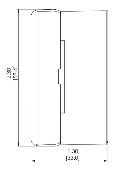
Tolerances: ± 0.02 in / 0.5 mm. All dimensions are in: inches [millimeters]
