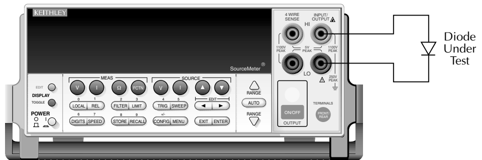
Figure 10-8 Connections for diode I-V tests
