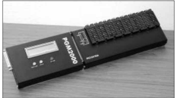
PGM2000 Master Control Unit connected to a PIC program adapter for stand-alone duplication
