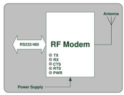
The RF modem can be configured to scan the radio link for activity and verify it is free before transmission thereby avoiding data collisions.
