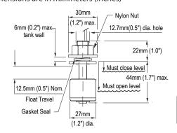
Thread sizes RSF53/4/6 M12x1.75 Thread Also available with 1/8" NPT Thread
