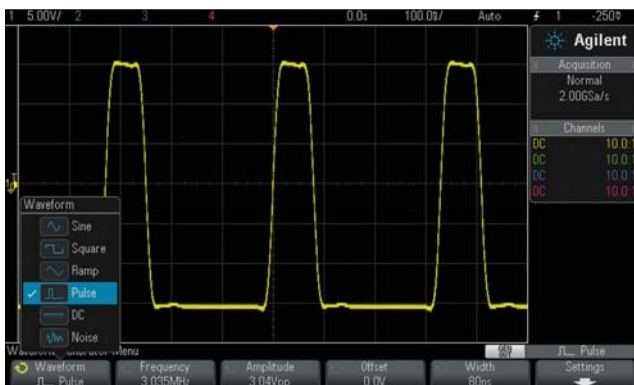
Figure 4: The WaveGen general-purpose function generator provides a built-in stimulus source for student experiments.
