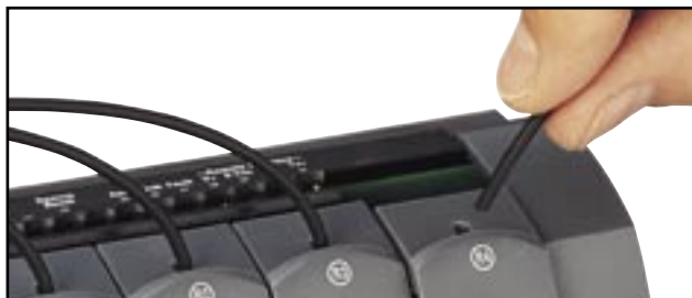
Figure 3-3. Installing the prepared fiber ends into the controller
