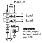
Contact Operation: Load contacts 3-4 & 5-6 open when the level rises to the short electrode connected to terminal 10. They close when the level recedes below the long electrode connected to terminal 7.
