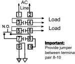
Contact Operation: Load contacts 3-4 & 5-6 open when the level recedes below the electrode. Then close when the level rises to the electrode and the normally open pushbutton switch is momentarily actuated.
