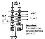
Contact Operation: Load contacts 3-4 & 5-6 close when the level recedes below the electrode. Then open when the level rises to the electrode and the normally open pushbutton switch is momentarily actuated.
