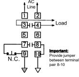
Contact Operation: Load contacts 3-4 close when the level rises to the electrode. It opens when the level recedes below the electrode and the normally closed pushbutton switch is momentarily actuated.
