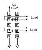
Contact Operation: Load contacts 3-4 open & load contacts 7-8 close when the level rises to the electrode. Contact 3-4 closes & load contacts 7-8 open when the level recedes below the electrode.
