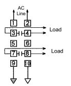
Contact Operation: Load contacts 3-4 & 7-8 close when the level rises to the electrode. They open when the level recedes below the electrode.
