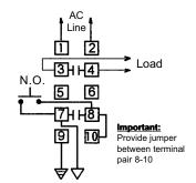
Contact Operation: Load contacts 3-4 open when the level recedes below the electrode. They close when the level rises to the electrode and the normally open pushbutton switch is momentarily actuated.
