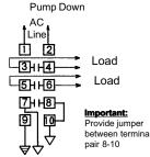
Contact Operation: Load contacts 3-4 & 5-6 close when the level rises to the short electrode connected to terminal 10. They open when the level recedes below the long electrode connected to terminal 7.
