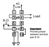
Contact Operation: Load contacts 3-4 close when the level recedes below the electrode. They open when the level rises to the electrode and the normally open pushbutton switch is momentarily actuated.
