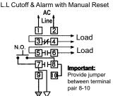
Contact Operation: Load contacts 3-4 close & 5-6 open when the level recedes below the electrode. Contacts 3-4 open & contacts 5-6 close when the level rises to the electrode and the normally open pushbutton switch is momentarily actuated.
