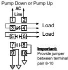
Contact Operation: Load contacts 3-4 open & contacts 5-6 close when the level rises to the short electrode connected to terminal 10. Contacts 3-4 close & contacts 5-6 open when the level recedes below the long electrode connected to terminal 7.
