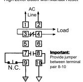
Contact Operation: Load contacts 3-4 open when the level rises to the electrode. They close when the level recedes below the electrode and the normally closed pushbutton switch is momentarily actuated.
