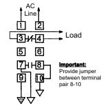
Contact Operation: Load contacts 3-4 open when the level rises to the short electrode connected to terminal 10. They close when the level recedes below the long electrode connected to terminal 7.
