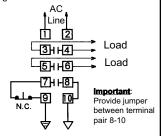
Contact Operation: Load contacts 3-4 & 5-6 close when the level rises to the electrode. Then open when the level recedes below the electrode and the normally closed pushbutton switch is momentarily actuated.
