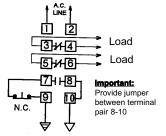
Contact Operation: Load contacts 3-4 & 5-6 open when the level rises to the electrode. Then close when the level recedes below the electrode and the normally closed pushbutton switch is momentarily actuated.
