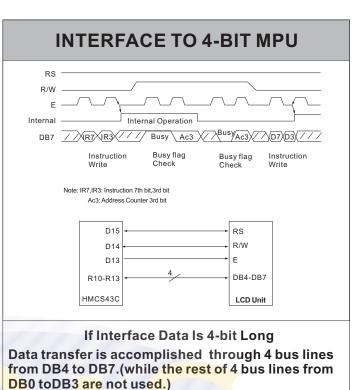
Data transfer is completed when 4-bits of data is transferred twice.(upper 4-bits of data, then lower
