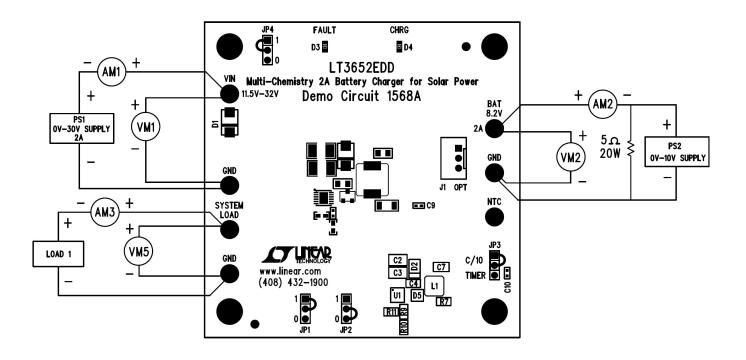
Note: All connections from equipment should be Kelvin connected directly to the Board PINS which they are connected to on this diagram and any input, or output, leads should be twisted pair.
