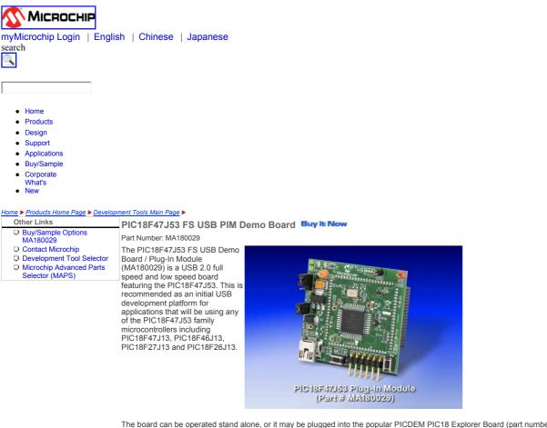
The board can be operated stand alone, or it may be plugged into the popular PICDEM PIC18 Explorer Board (part number <u>DM183032</u>) for additional functionality. When the board is used in the stand alone configuration, the included RJ-11 to ICSP adapter (part number <u>AC164110</u>) can be used to reprogram the board using RJ-11 based programmers.
