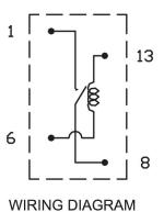
MVS7 must be mounted veritcally. Pin #1 is up.
