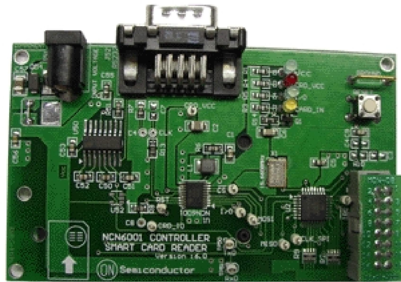
through a simple and flexible micro controller interface. On top of that, thanks to the built in chip select pin, several couplers can be connected in parallel. The device is particularly suited for low cost, low power applications, with high extended battery life coming from extremely low quiescent current.
