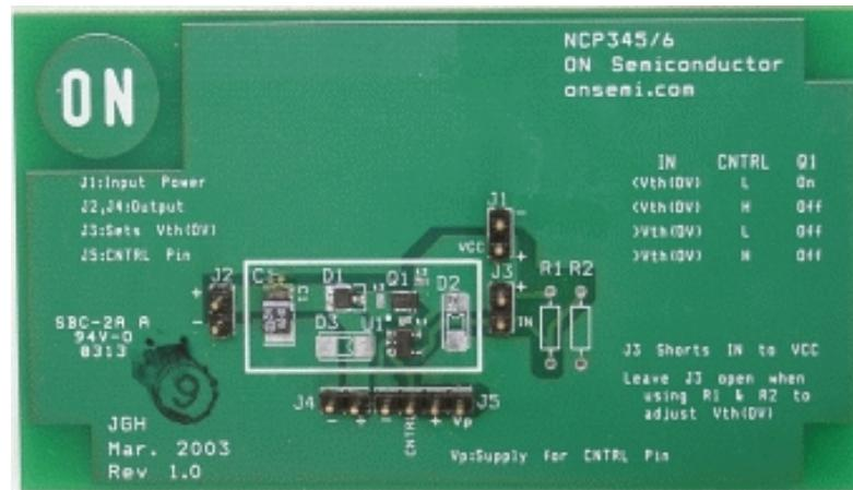
supply faults when used in conjunction with an external P -channel FET. The device is designed to sense an over voltage condition and quickly disconnect the input voltage supply from the load before any damage can occur. The OVP consists of a precise voltage reference, a comparator with hysteresis, control logic, and a MOSFET gate driver.
