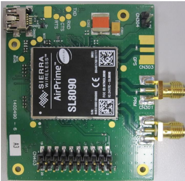
Figure 59. Configuration of the AirPrime SL80xx Socket-Up Board for Current Consumption Measurement
