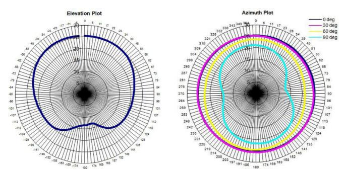
The strength of the PowerHelix antenna technology is its immunity to de-tuning in the presence of dielectric loading, like human tissues. The SL1206 antenna retains efficiency and polarization near the human body. Conventional antennas lose 5-10dB of gain in similar circumstances.
