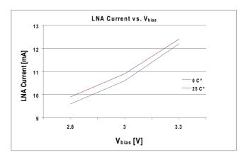
The SL1206 high-gain, low-noise amplifier, optimized for 3Vdc, provides 25dB peak gain with less than 1.25dB insertion loss at a current draw of less than 14mA.
