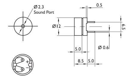
**Dimensions** Unit: mm Tolerance: ±0.5mm
