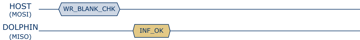
Figure 21 – Command WR_BLANK_CHK (erased state)
