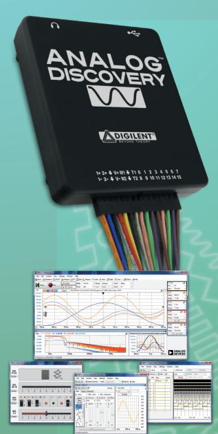
Turn your PC into a powerful circuit learning platform that can measure, visualize, analyze, record and control mixed signal circuits! The Analog Discovery is small enough to fit in your pocket and costs less than a textbook, but it is powerful enough to replace a stack of lab equipment. Powered by a Hi-Speed USB port and the free WaveForms software, the Analog Discovery lets you build and test analog and digital circuits outside of the lab.
