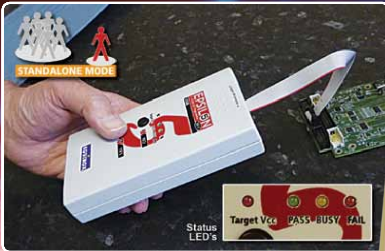
The EPSILON5 MK IV programmer being used in standalone mode
