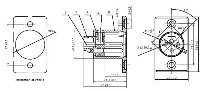
The pin plating gold, thickness 0.05µm (SOLDER).
