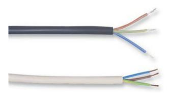
Description : Circular 3-cores, 1.5 mm<sup>2</sup> (30 / 0.25 mm) tinned copper, 150°C silicone rubber insulated, laid up, 85°C PVC
