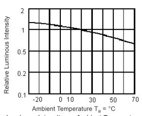
Luminous Intensity vs. Ambient Temperature
