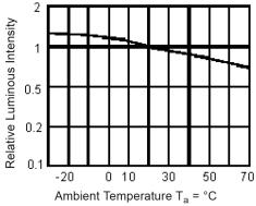
Luminous Intensity vs. Ambient Temperature
