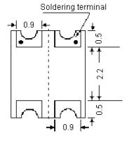
Recommended Soldering Patten for Reflow soldering
