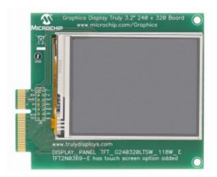
The Graphics Display Truly 3.2" 240x320 Board is a demonstration board for evaluating Microchip's graphic display solution and graphics library for 16- and 32-bit microcontrollers. It is an expansion board compatible with the PIC24FJ256DA210 Development Board (DM240312), and Graphics LCD Controller PICtail™ Plus SSD1926 Board (AC164127-5). The features include:
