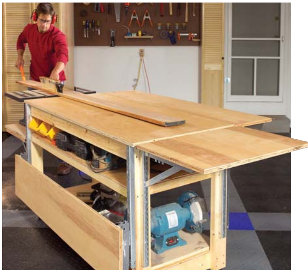
Locking casters make this bench mobile. It also has a low shelf at one end that allows the bench to double as an outfeed table for a table saw. Shelf hardware makes it even more adaptable.
