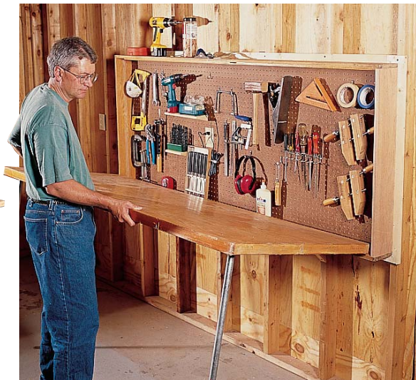
A classic workbench for small shops is one that folds down from the wall. This one uses a solid-core door for a top, and 1-1/2-in. pipe for legs. The pipes screw into pipe flanges on the door.
