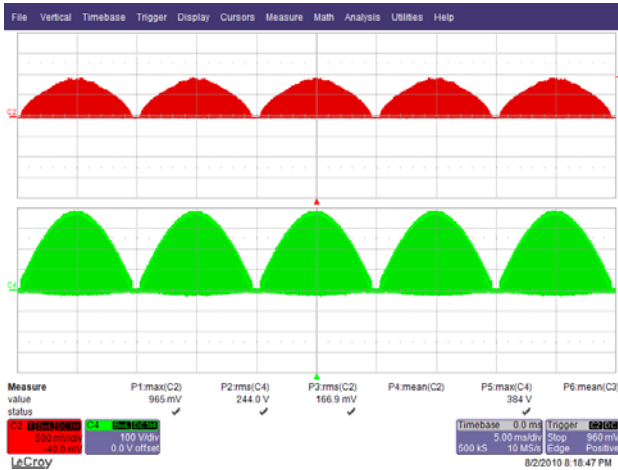
Figure 24 – 265 VAC 50 Hz, Full Load. Upper: I_{DRAIN} , 500 mA / div. Lower: V_{DRAIN} , 100 V, 5 ms / div.
