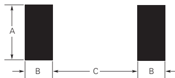
Figure S13 Recommended Pad Layout for Surface-mount Devices
