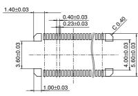
Recommended metal mask pattern Metal mask thickness: When 150 µm (Terminal portion opening area ratio: 53%) (Metal portion opening area ratio: 100%)
