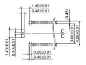
Recommended metal mask pattern Metal mask thickness: When 120 μm (Terminal portion opening area ratio: 66%) (Metal portion opening area ratio: 100%)
