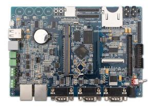
MBS-SAM9X25 SBC board operates at up to 400MHz, with 256 Mbytes NandFash ,128MB DDR II,4MB serial DataFlash and 64KB serial EEPROM. It supports Linux 2.6.39 ,offer angstrom and android-2.3.5\_r1 test .The board provides a wide range of peripherals, including a high-speed USB2.0 port(480MHz), an Ethernet 10/100M interface, audio interface, a JTAG debug port,Micro SD card interface,SD/MMC card interface, CMOS camera interface.It supports video data collection.
