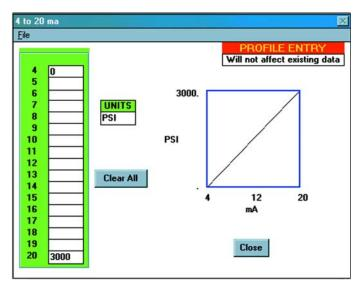
Click the scale button in the file menu to create custom scales and engineering units for DC voltage (Models L410 & L430) and DC current loggers (Model L320).
