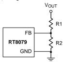
Figure 1. Setting the Output Voltage
