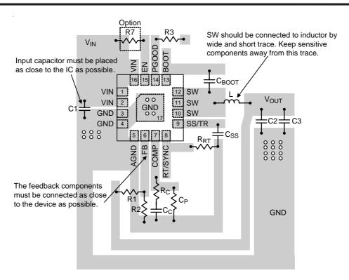
Figure 3. PCB Layout Guide
