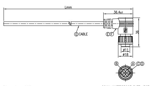
Dimensions : Millimetres CONN. WATERPROOF RATE: IP67
