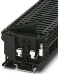
Fuse terminal block for cartridge fuse insert, cross section: 0.2 - 4 mm 2 , AWG: 26 - 10, width: 8.2 mm, color: black
