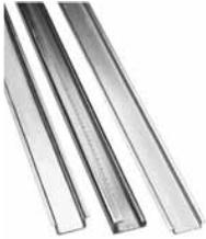
DIN Type Rails receive terminal blocks, relays, switches, filters, timers and various other electrical and electronic components manufactured by European, Japanese and U.S. firms. Available in three styles: (1) asymmetric, DIN 1 profile; (2) symmetric, DIN 3 profile; (3) heavy-duty CENELEC profile. All DIN rails are 78.74-in. (2000-mm) long and plated.
